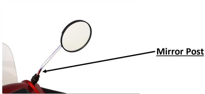
To attach the mirrors simply place each mirror threaded end into the mirror post. Turn mirror clockwise and fasten mirror to scooter. Secure using a 14mm wrench on the mirror securing nut.
